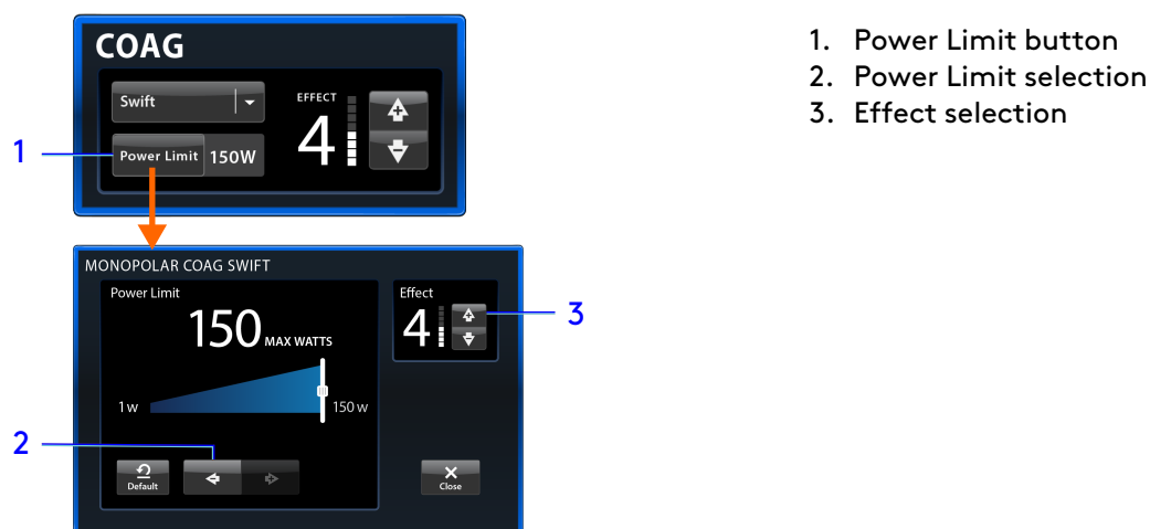
Figure 6.12 Power limit settings, Monopolar COAG example
