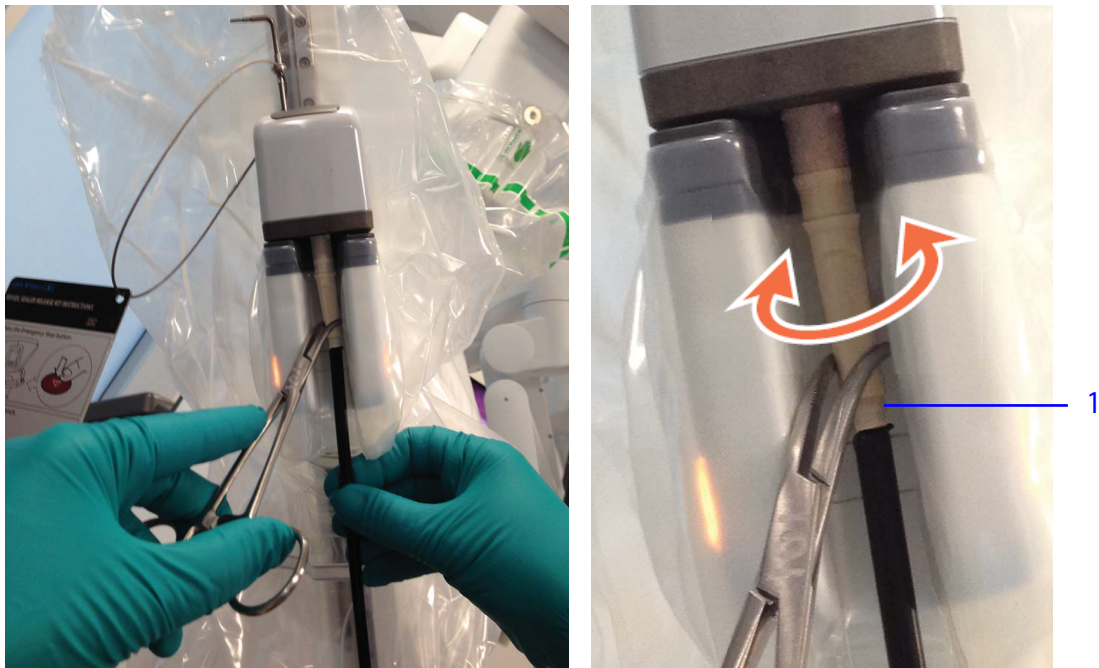
Figure 2.6 Using forceps, twist the roll gear while holding the shaft in place
