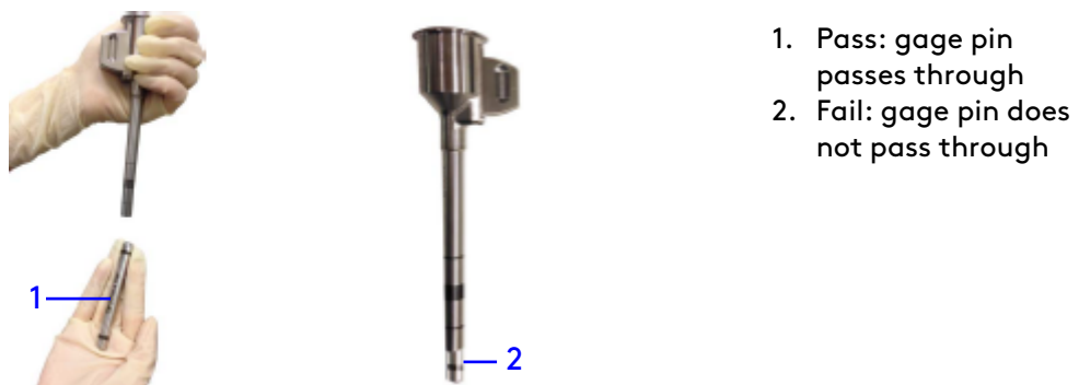
Figure 11.9 Gage pin pass and fail examples
