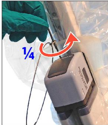
Figure 2.4 Keep the grip release tool engaged while manually opening the grips
