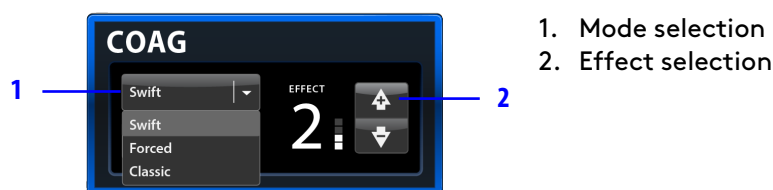
Figure 6.11 Mode and effect settings, Monopolar COAG
