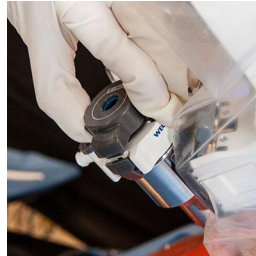
Figure 11.20 Correct reducer and cannula seal attachment
