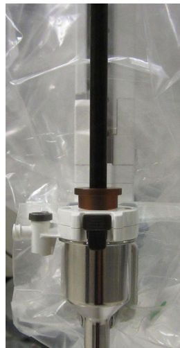
Figure 2.10 Sliding the instrument introducer down the shaft before instrument removal
