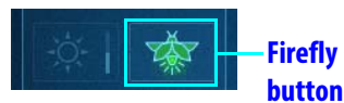
Figure 4.5 Surgeon Console Firefly button on endoscope arm pod, icon is completely lit green in Sensitive mode
