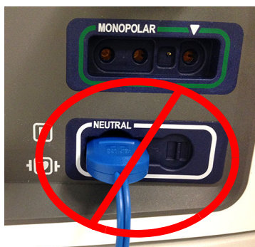
Figure 8.12 Do not connect the patient neutral pad directly to the VIO dV
