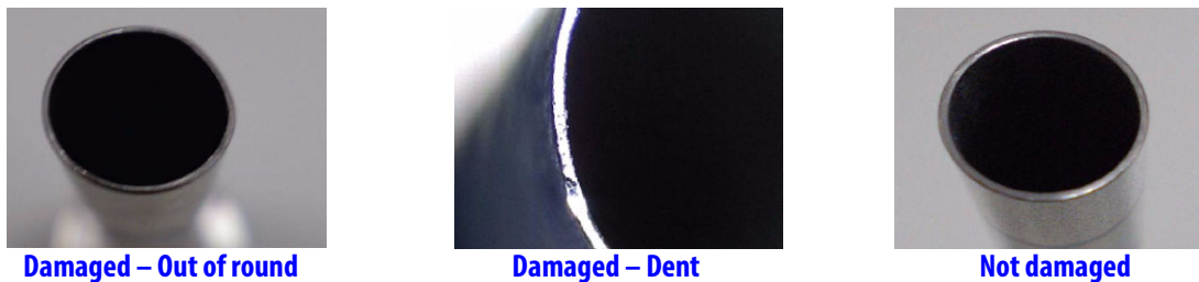
Figure 9.5 Visual inspection examples
